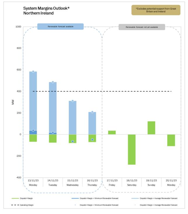
When a negative dispatch margin coincides with a low renewable generation forecast, the net renewable generation value may appear below the zero axis (low forecast: •, average forecast: •). It should be noted that the Daily Dispatch Margin and renewable generation forecast are highly variable. The outlook is based on **estimates** and is therefore subject to rapid changes.
